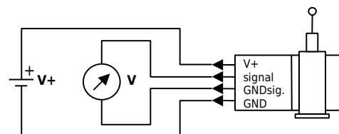
note: GND sig. and GND may be connected in 3-wire system.
