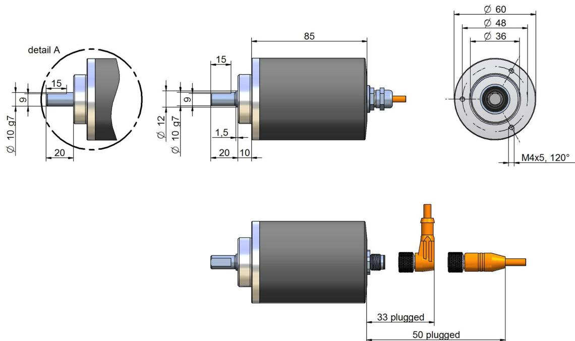
Note: „detail A“ is valid for all rotary transducers with a measurement range of 15 turns or more!
